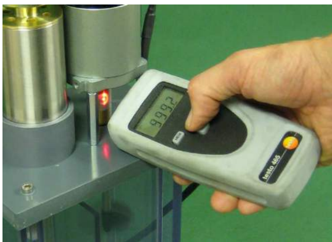
Fig. 6.4 Checking the impeller speed by means of an optical tachometer.
